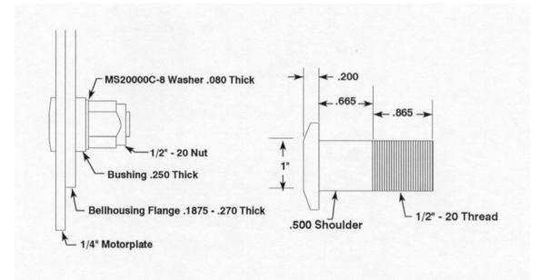
B. The motor plate stud (1/2", 12.7mm) must be a minimum of Grade 5 and fabricated per the drawing above. Certification of mechanical properties and identification of the stud manufacturer must be on file with SFI. The stud hole must have a 1/4 inch (6.4mm) thick bushing, tack welded to the bellhousing flange with a minimum outer diameter of 3/4 inch (19mm).
